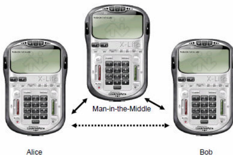
Figure 5: Setting of Man-in-the-Middle Attack. All clients are assumed to be in the same local network.
