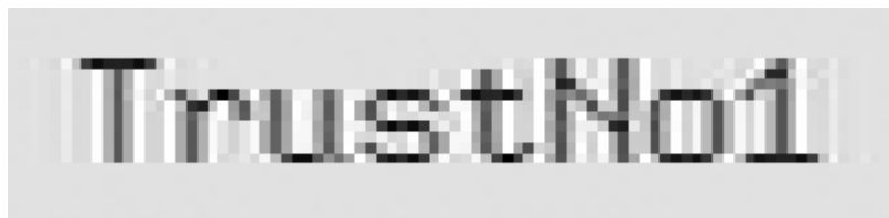
Figure 2: The same text after horizontal low-pass filtering.
